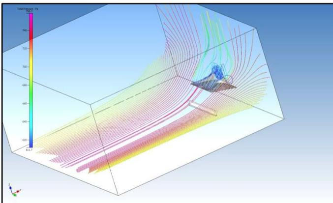
Figure Nine: Higher Level Particle Trace highlighting the wind turbulence effect onto the face of the building. This style of visualization assists the building designer to compensate for the additional stress transfer to the building supports.
