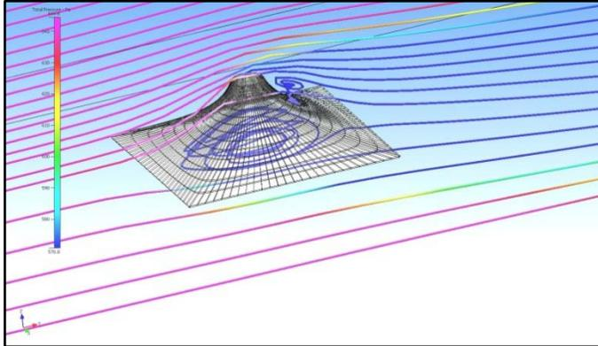
Figure Five: Free Standing square based single conic with Bail Ring closed. Particle Trace from CFD software showing wind turbulence over a conic profile with closed bail ring.
