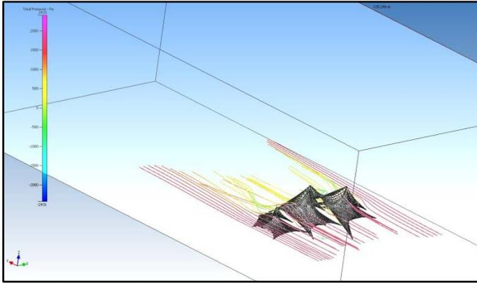
Figure Fifteen: Particle Trace highlighting wind turbulence within a multiple sail configuration.
