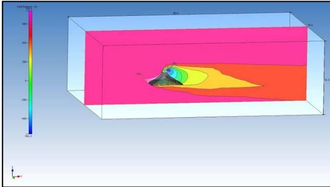
Figure One: Free Standing Square based single Conic with bail ring open . Visualization slice from CFD software showing wind simulation over a conic profile with open bail ring.
