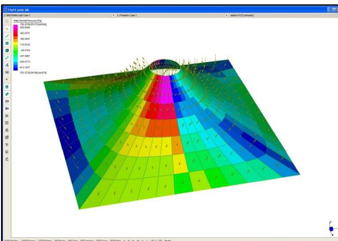
Figure Three: FEA Model of Free Standing Square based Single Conic. Utilizing the FSI the CFD simulation results are pressure mapped directly onto the canopy profile within the FEA package ready for analysis.
