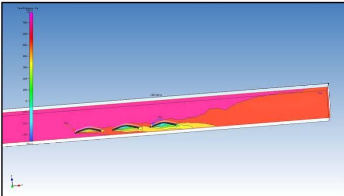
Figure Eleven: Multiple Configuration Barrel Vault Car Park Structures. Visualization Slice illustrating the wind effect in a multiple structure configuration.
