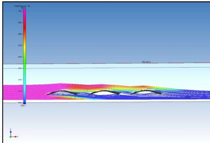
Figure Twelve: Particle Trace illustrating the influence multiple structures have on the downwind landscape.
