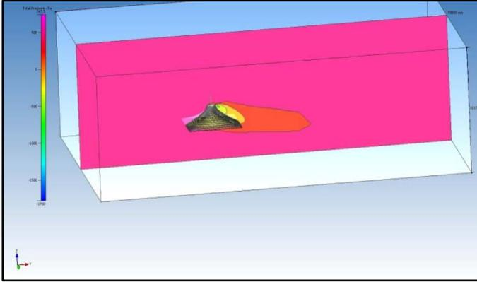
Figure Four: Free Standing Square based single Conic with bail ring closed. Visualization slice from CFD software showing wind simulation over a conic profile with closed bail ring.
