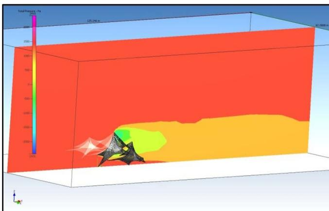
Figure Fourteen: Visualization Slice of 318 sq mts of PTFE tensile sails covering an outdoor recreation area in the UAE. The wind influence multiple structures have on the surrounding landscape is highlighted.
