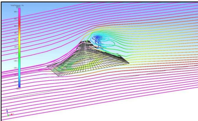
Figure Two: Free Standing Square based single Conic with bail ring open. Particle Trace from CFD software showing wind turbulence over a conic profile with open bail ring.
