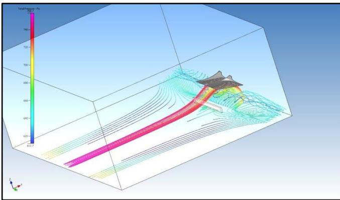
Figure Eight: Particle Trace Visualization highlighting wind turbulence generated along lower level front exterior. Large buildings significantly affect airflow and influence ground level wind speeds around their base. This can lead to the development of very high wind speeds around the base of a building, rendering certain areas unsafe for pedestrians. On a smaller scale, moderate wind speeds may make areas uncomfortable and therefore unsuitable for a street café.
