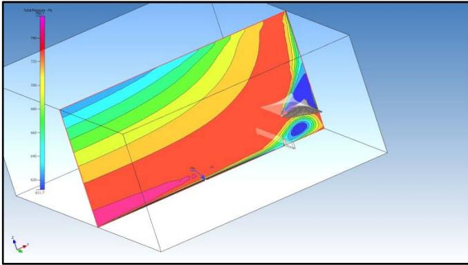
Figure Seven: Visualization Slice illustrating the high and low pressures generated by wind and topography influence on the double conic structure, building and surroundings.
