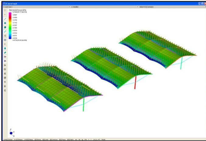
Figure Thirteen: FEA Model of multiple Barrel Vault structures. Pressure mapping applied from CFD simulation allows for accurate nomination of structural steel supports and foundation detail thus alleviating the issue of either over compensating or underestimating design criteria.
